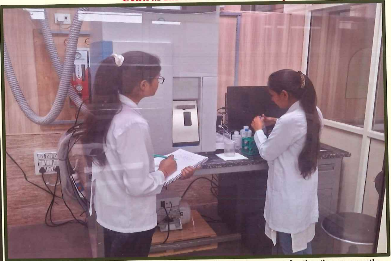
The post graduate students of the university performing heavy metal estimation on recently upgraded Inductively coupled plasma mass spectrometer in central instrumentation facility
